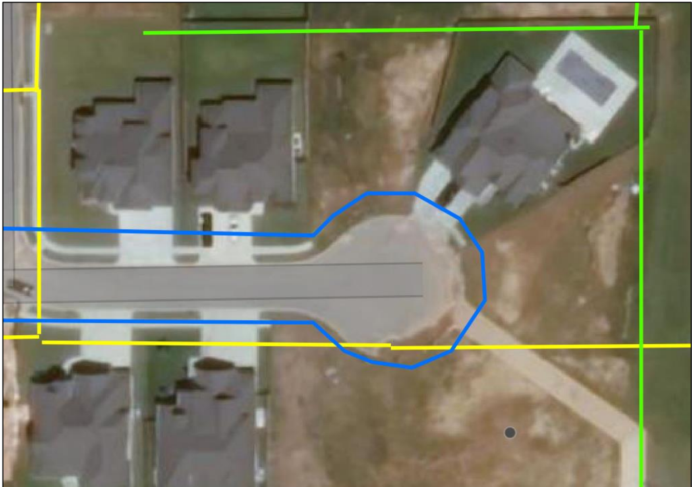
Figure 1: Utility Lines | Sewer-green, Water-blue, Storm water-yellow
