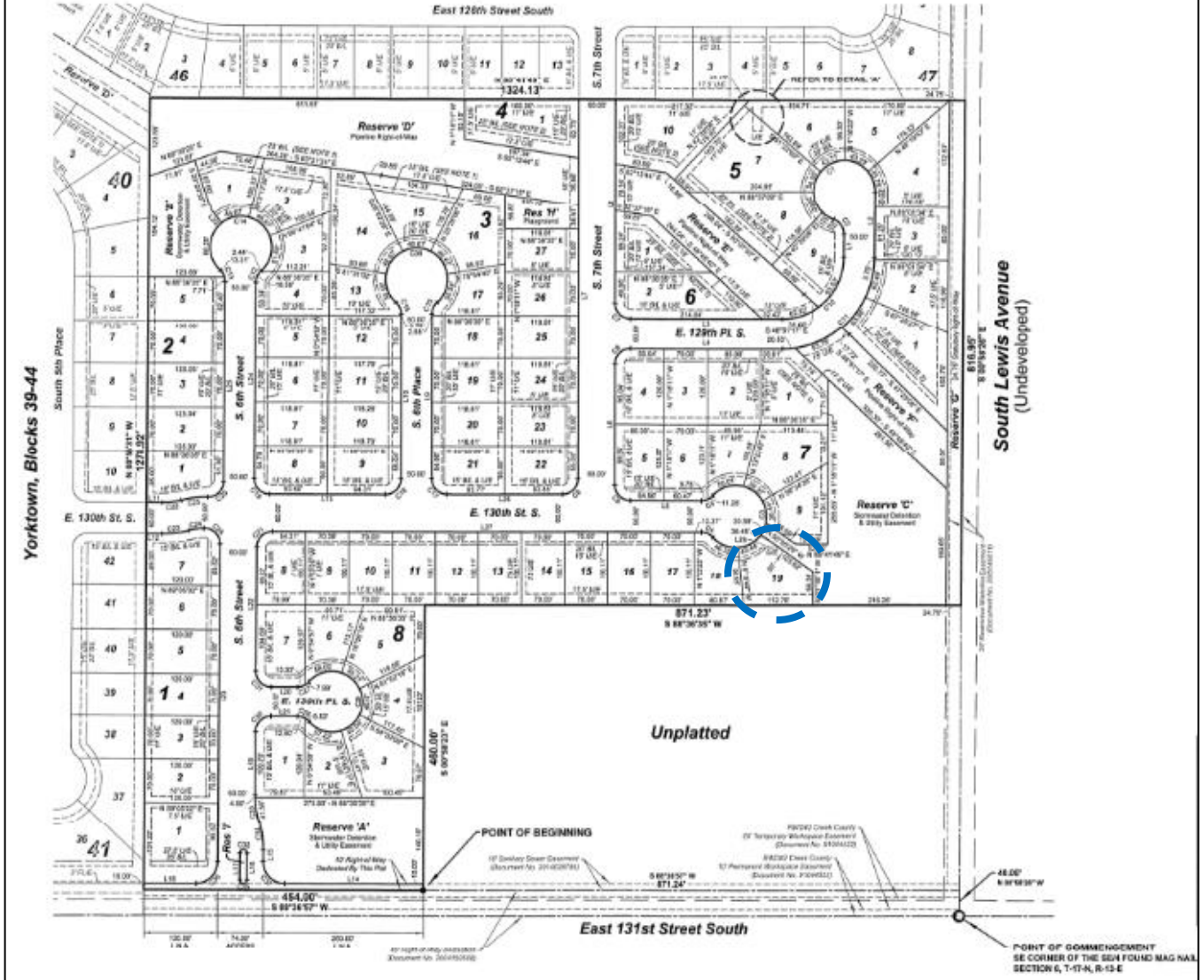
Figure 2: Plat drawing with adjacent Drainage Easement identified
